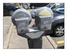
By converting the dual meter housings to single meters, the coin capacity of each meter pole is doubled. Since each meter has its own coin canister, the increased coin capacity will reduce the frequency of meter collections.
